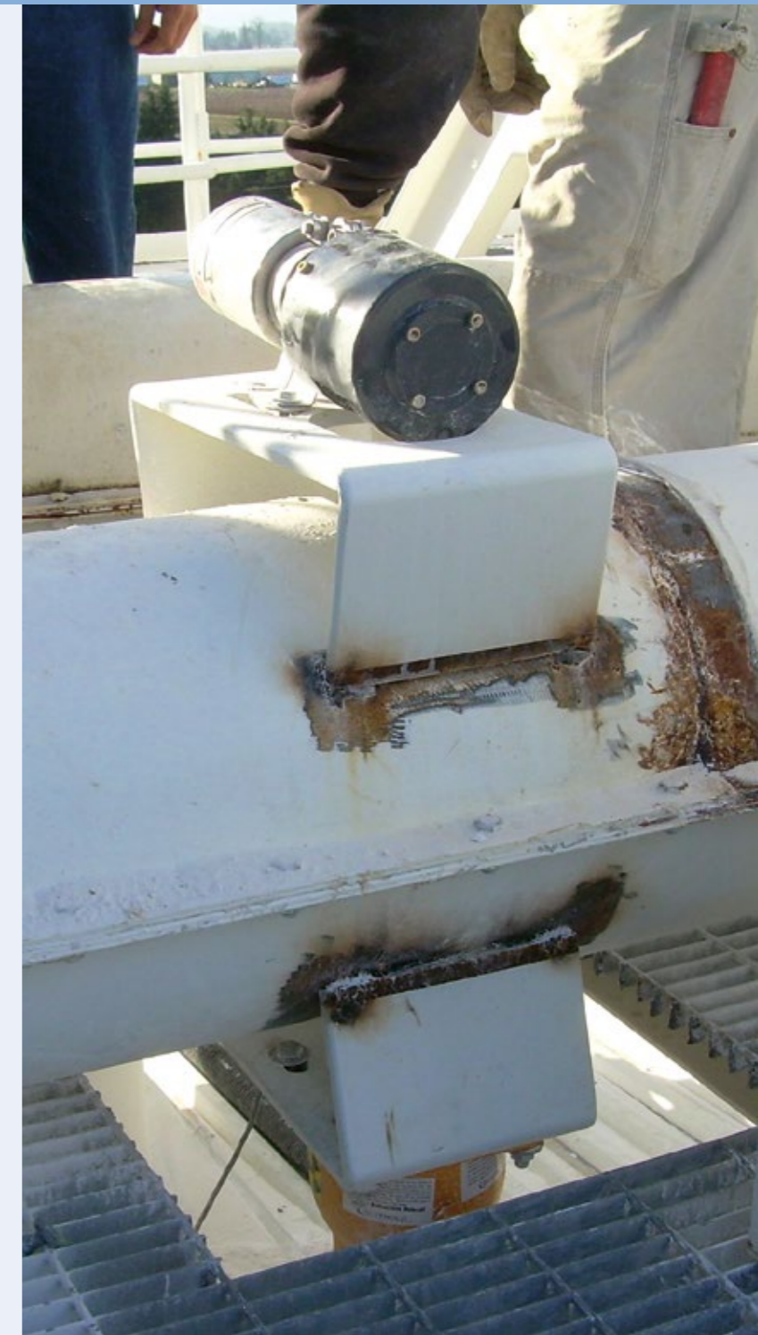
Bulk flow measurement on a screw conveyor
